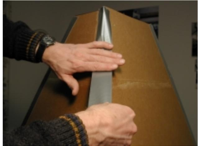
7. Finish the last joint inside the reflector by applying the remaining piece of duct tape.
