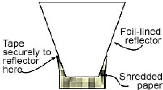
Insulate the box below the reflector using shredded newsprint.
