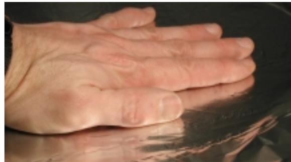
Smooth out the foil carefully, removing any wrinkles or bubbles as you go.
