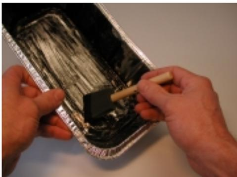
Use two coats of black paint to coat the inside of the baking chamber.
