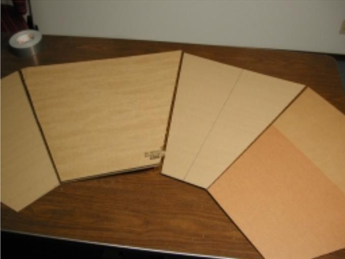
3. Carefully position the first two panels, keeping a 2 mm space between them. Position one of your 60- cm strips of duct tape over the joint between the panels. Press it onto the joint, being sure it sticks securely to both panels over its full length.
