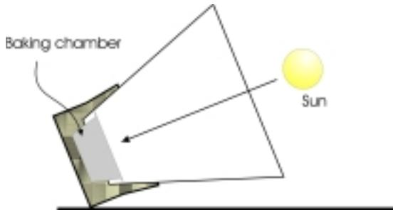
Position the oven so that the baking chamber faces the sun squarely and the shadow of the reflector is minimized.
