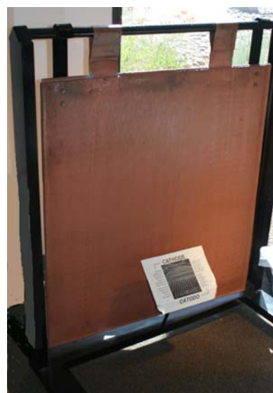
Figure 2. A copper cathode consists of 99.9% pure copper
