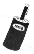
Use a piece of paper towel to wide any electrolyte mix off of the graphite rod.
