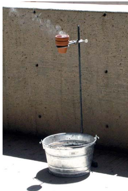
Figure 1. Apparatus for the thermite reaction.
