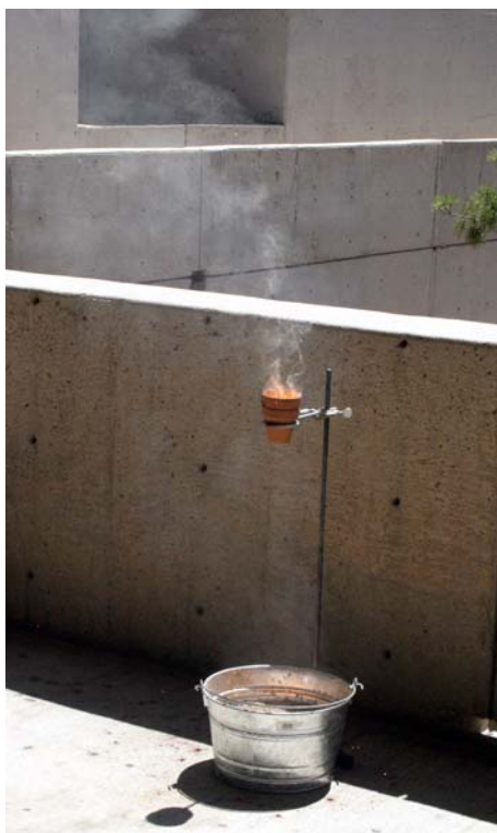
Figure 5. The reaction is just completed. Note that the inside of the flower pot is glowing red and the reflection of the molten iron is visible in the bucket.
