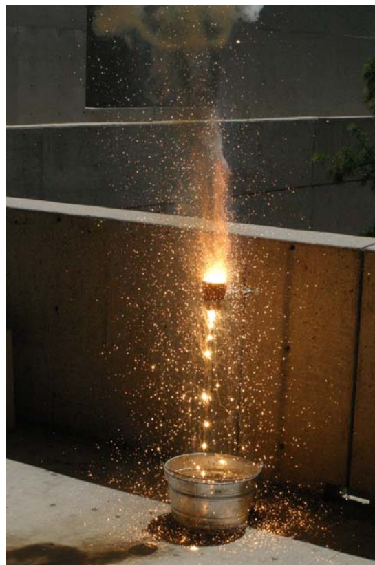
Figure 4. Molten iron falling from the flower pots into the sand.
