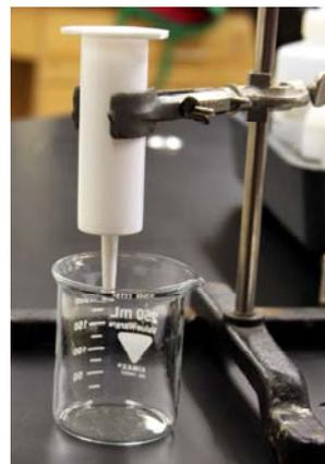
Remove the plunger from the extractor. If the cotton moves up the Extractor tube, use a glass stirring rod to push it down to the bottom. Slowly pour the prepared sample solution in the 250 mL beaker into the extractor.
