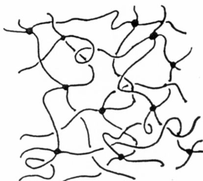
Figure 3. Schematic sketch of a typical elastomeric network
