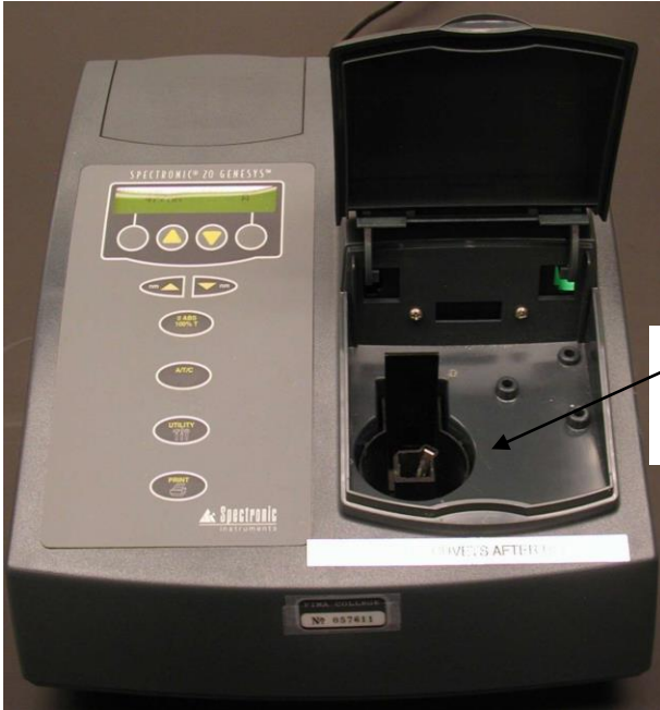
Figure SP-3. The Spectronic 20 with the light shield raised showing the cuvette holder.
