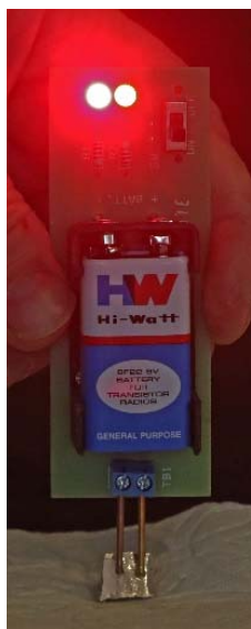
Figure 3. The conductivity of sodium metal. Photo by David A. Katz
