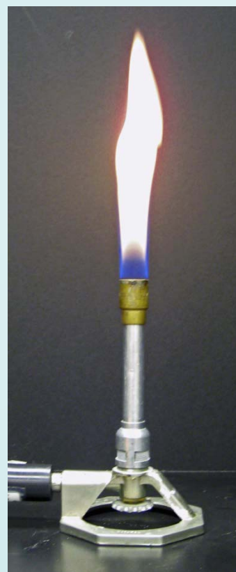
Incorrect flame adjustment
