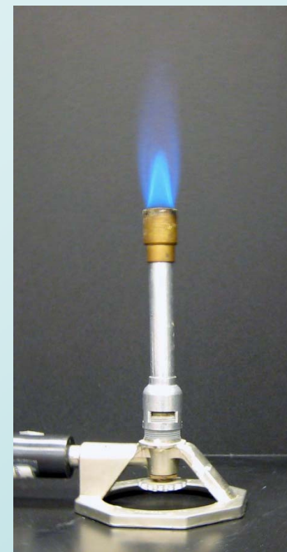
Properly adjusted flame
