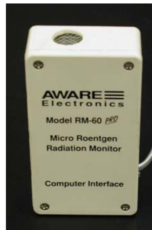
Figure 1. Aware Electronics Model RM-60 Geiger tube.
