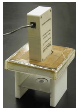
Figure 2. Geiger tube with stand.
