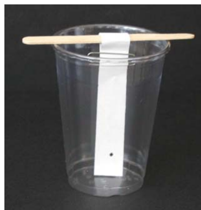
Figure I-3. Chromatography of a thin strip of paper for single ink samples.
