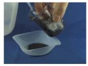
Transfer the solid to a weighing boat with the aid of a few squirts from a wash bottle.
