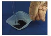
Add 1-2 mL of 25% tetramethylammonium hydroxide. Gently stir with a glass rod for at least a minute to suspend the solid in the liquid. Use a strong magnet to attract the ferrofluid to the bottom of the weighing boat. Pour off and discard the dark liquid. Move the strong magnet around and again pour off any liquid. If the ferrofluid does not spike, continue to move the strong magnet around, pouring off any liquid.
