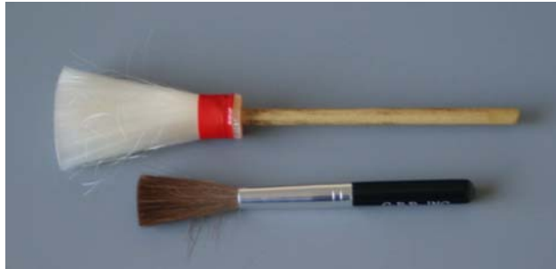
Figure F-4. Fingerprint brushes. A fiberglass brush (top) and a camel hair brush (bottom).
