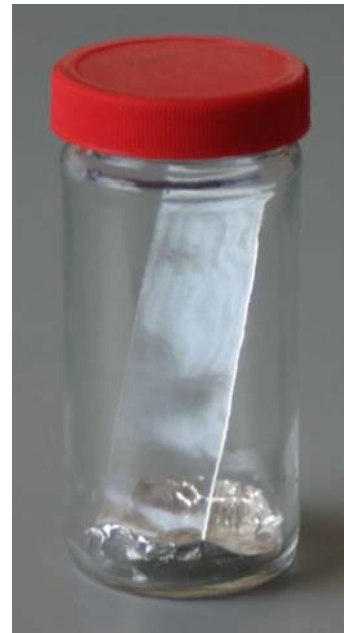
Figure F-5: Superglue development of a fingerprint on a microscope slide in a spice jar
